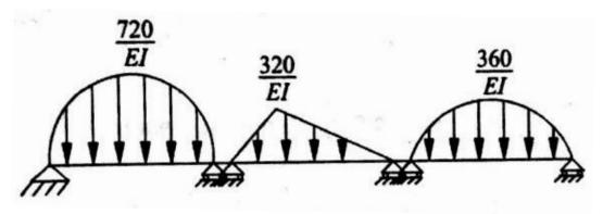
The maximum ordinate of load in AB =  $\frac{1}{EI} * 40 * \frac{12^2}{8} = \frac{720}{EI}$ The maximum ordinate of load in BC =  $\frac{1}{EI} * \frac{120*4*8}{8} = \frac{320}{EI}$ The maximum ordinate of load in CD =  $\frac{1}{EI} * 20 * \frac{12^2}{8} = \frac{360}{EI}$
